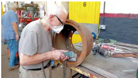
Cardiff 262's inner brake drum surface being manually blended. [Keith Walker]
